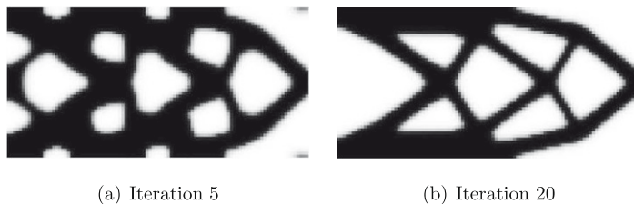
Fig. 9. Optimal configurations of the cantilever example on a coarser 100 \times 50 mesh at iterations 5 and 20.
